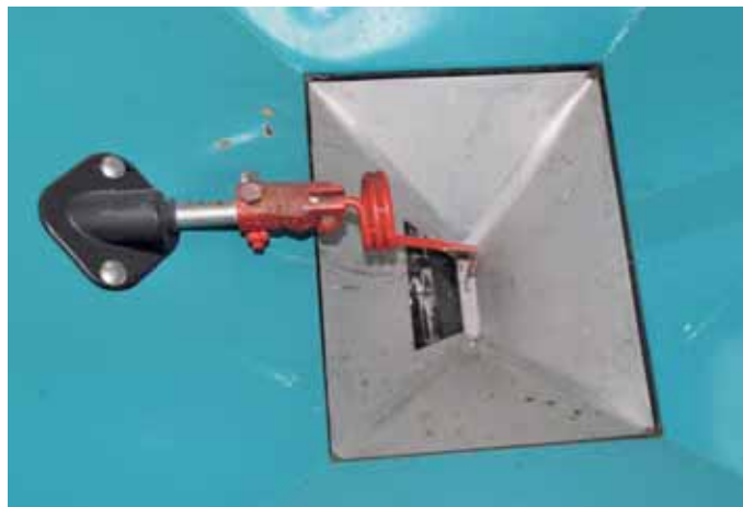
The oscillating finger remedies any clumps or inadequate pouring of the fertiliser.
