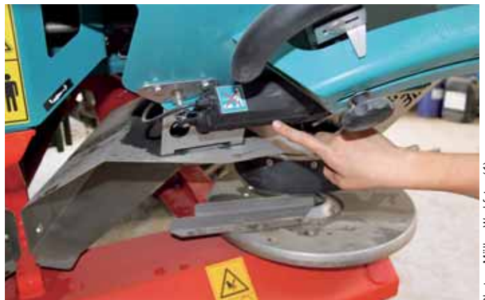
The fertiliser spreader hangs in a weighing frame with a 10 tonne load cell. In the case of the weighing distributor, an electric actuator adjusts the distribution amount according to the speed and trickle ability.
