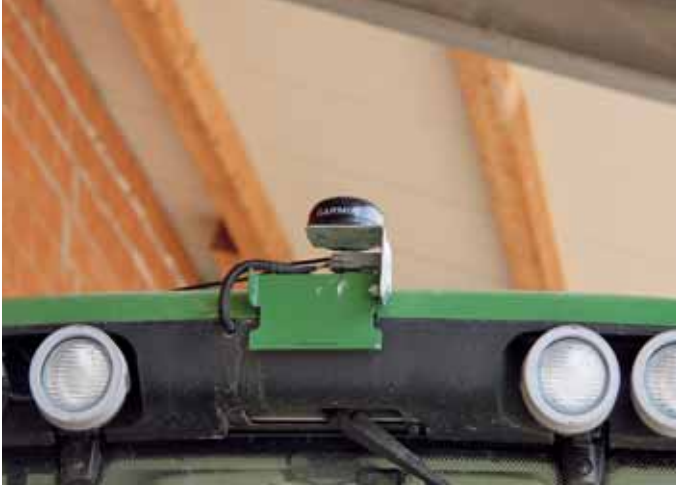
Via the GPS antenna, the Vision X computer receives a very precise speed signal although there is a slight delay.
