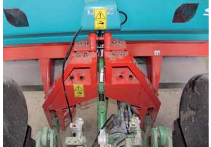
The distributor hangs in a weighing frame with a 10 tonne load cell.
