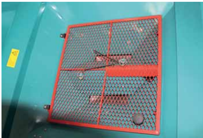
The sieve prevents the clotted fertiliser from falling into the Hopper base.
