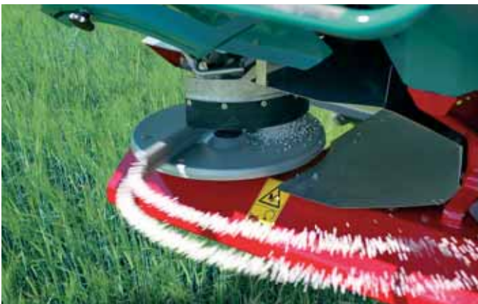
The fertiliser from every swing shovel is distributed through the epsilon shape in two trajectory streams. This should improve the accuracy of distribution.
