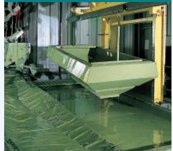
An important stage in the new SULKY anti-corrosion treatment process : all components are dipped by robot into a bath of paint primer.
